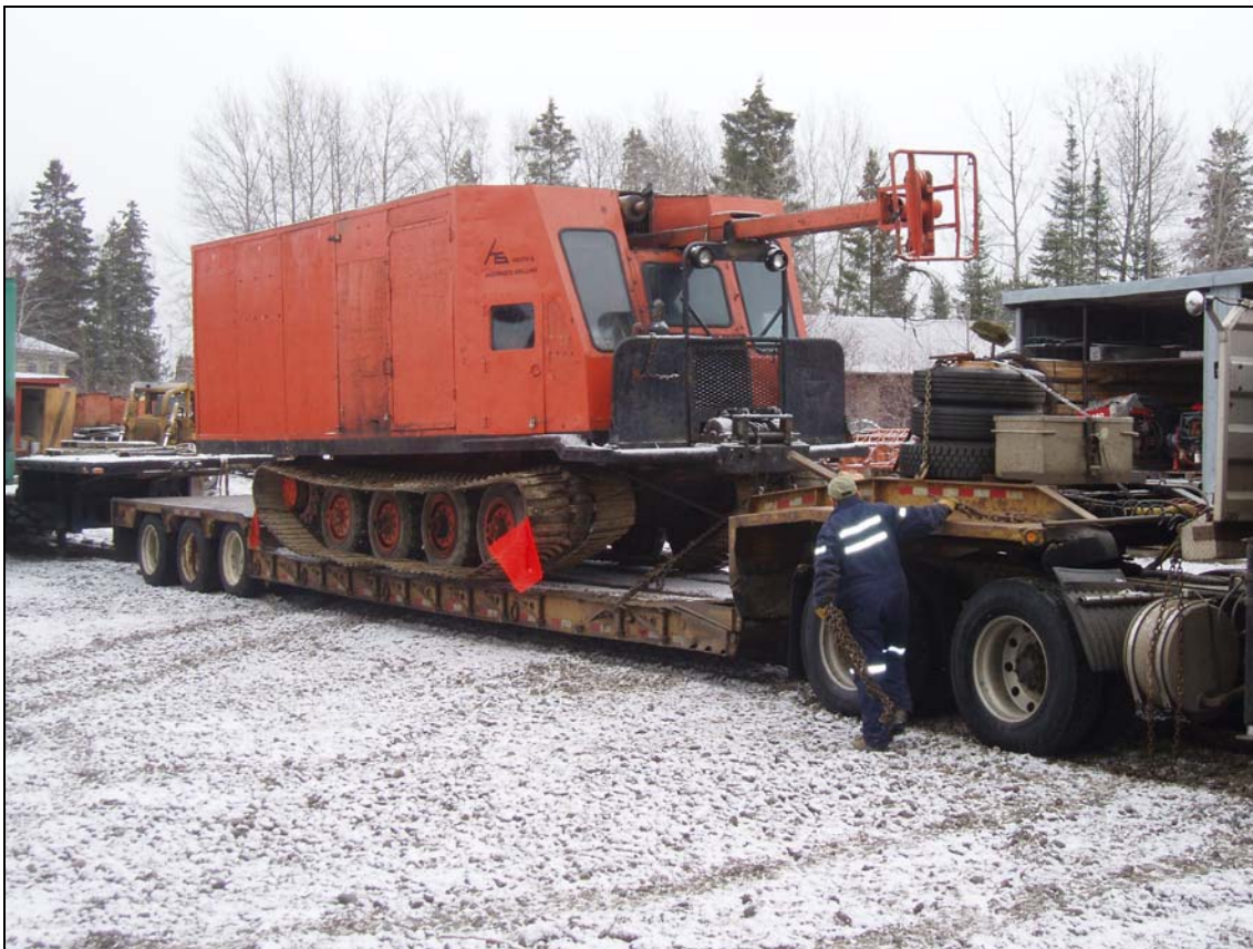
Figure 3 RC drill rig, prepared for truck transport at Cabo's Kirkland Lake Division. (Loeb Aron & Co. Ltd photo 2006)
